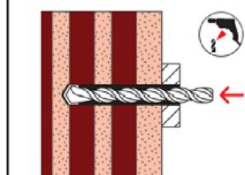
1. Drill the bore hole as per Table B2.1 using the drilling method described in the corresponding Annex C.
