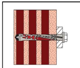
5. Correctly installed anchor.
