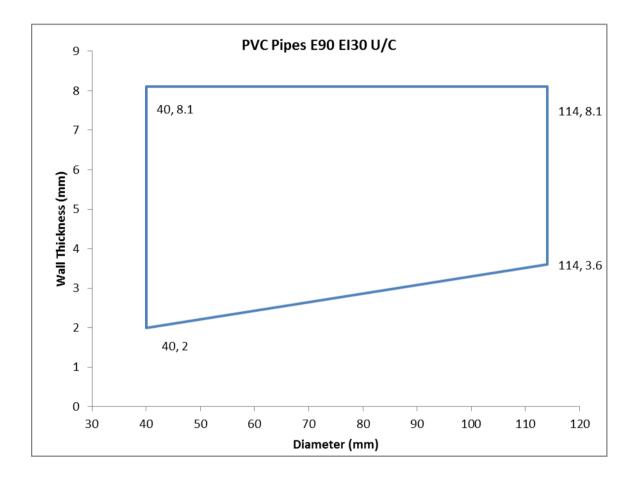
C.5.1 Rigid floor constructions according to 1.2.1 with wall thickness of minimum 150 mm incorporating Fischer FCPS Coated Panel System
